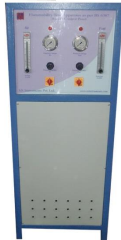
Burner Control Panel
